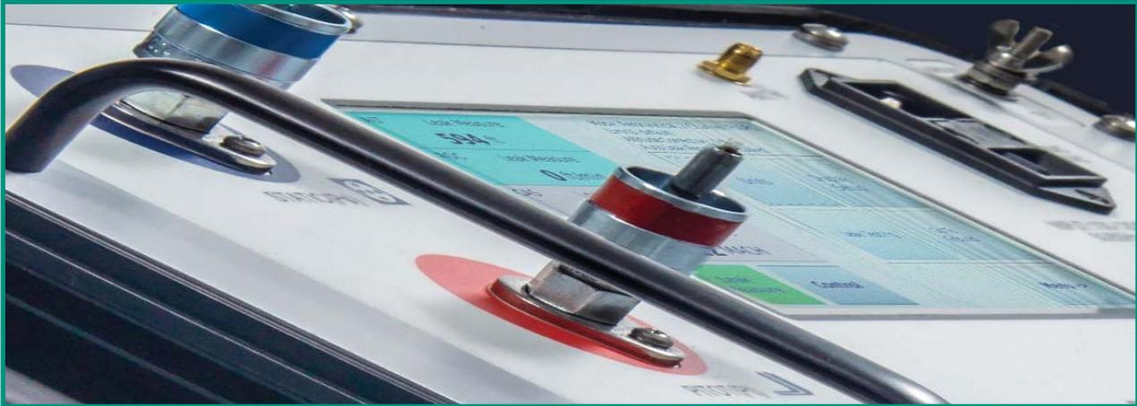
The DPS1000 performs altimeter and static systems tests and inspections. Critical components used in the DPS1000 have a well established history of proven flight line reliability & accuracy - including case, pumps, valves, and static/altitude transducers. Barfield introduces an innovative option to the DPS1000, wireless communication for display and control using the latest Wi-Fi technology.
